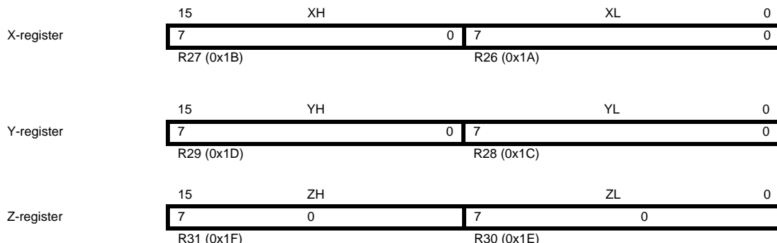
Figure 6-3. The X-, Y-, and Z-registers
